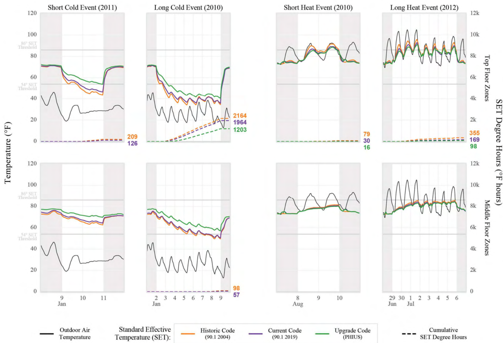
Figure F-20. New Multifamily: Atlanta, GA (3A)
